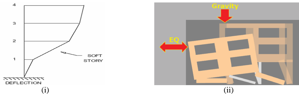
Fig.1 (i) Lateral displacement diagram of a building with a soft storey under lateral loading (ii) Collapse mechanism of a building structure having a soft storey.
